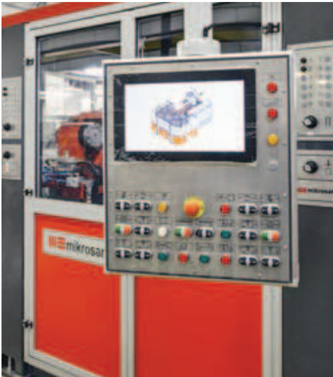
Injection blow molding machine automated by B&R and mapp Technology.
