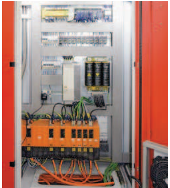
An extruder requires particularly efficient energy management to operate profitably. Mikrosan achieved exceptionally low energy consumption using ACOPOS-multi servo technology featuring active power regeneration.
